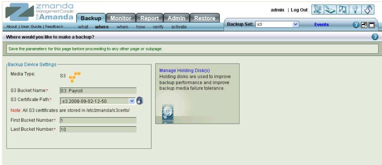
Figure 1. Choosing S3 as a backup target is as simple as selecting and naming an S3 “bucket” name.
